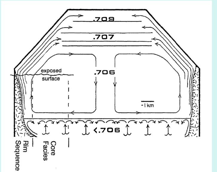
Fig 5. Model of evolution for a steep-walled magma chambe in which crystallization from the walls and roof produces more\_ buoyant fractionated liquids (McBirney and Baker, 1981).
